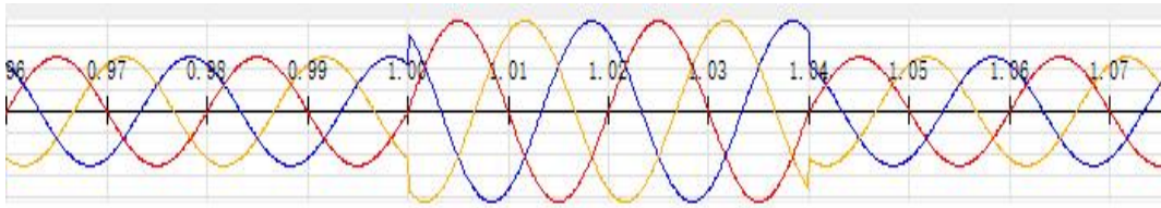
Figure 4.2.2.3.9.1 Waveform Screenshot of Voltage Swell
