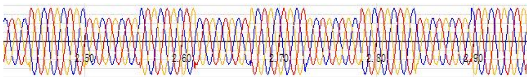
Figure 4.2.2.3.8.1 Waveform Screenshot of Voltage Flicker
