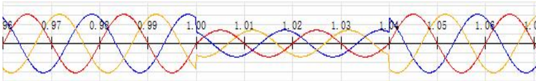
Figure 4.2.2.3.9.2 Waveform Screenshot of Voltage dip
