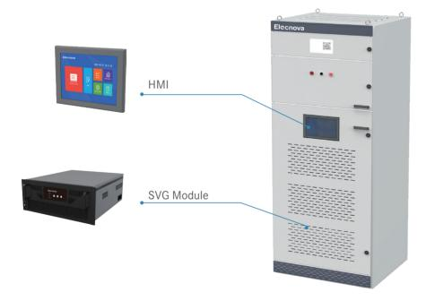
SFR-SVG is a new-generation product of Static Var Generator(SVG), it used the latest technology application for the reactive power compensation. When the SFR-SVG parallel in the grid, it equalized as a dynamic reactive current source. The reactive current of the SVG could be flexibly controlled and compensate the reactive power automatically.
