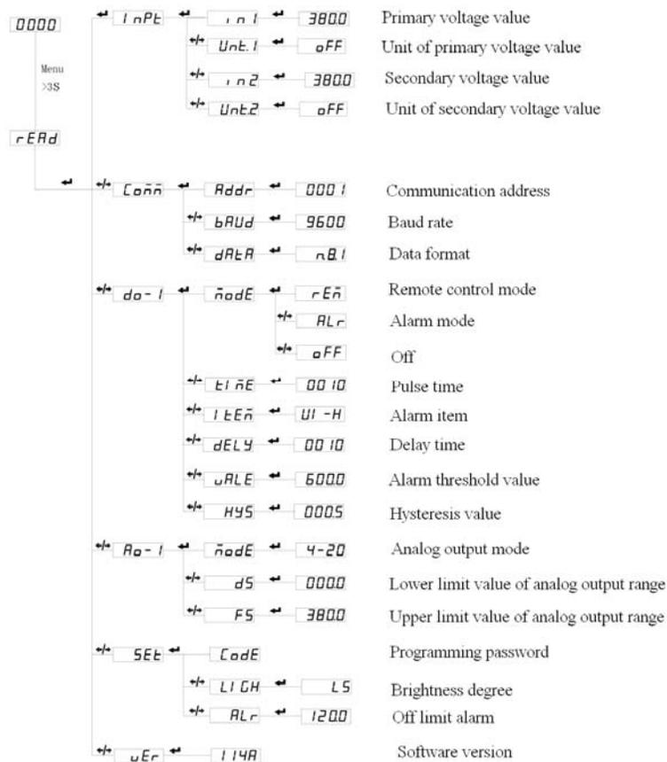
Figure 1. System parameter checking interface of single phase voltmeter
