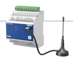
Rail-mounted intelligent multi-functional power meter PD194Z-E14C (GPRS), PD194Z-E14D (NB-IoT), PD194Z-E20C (GPRS), PD194Z-E20D (NB-IoT) have comprehensive power parameter measurement, complete power metering, and power quality analysis functions. The built-in wireless module enables wireless transmission of the power grid data.
