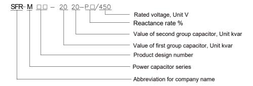
Note: total compensation for rated voltage 480V(P7) or 525V(P14), and separate compensation for rated voltage 280V(P7) or 300V(P14).
