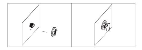
Installation method 2 (used for cut-out size 91×91mm,76×76mm,67×67mm)
