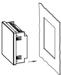
**Install the meter from the outside of the panel into the mounting hole.**
